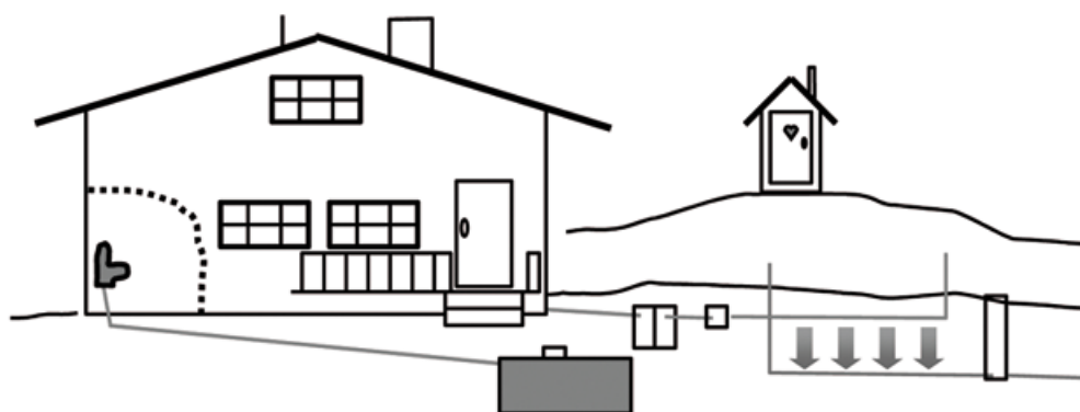
Figure 4. A solution in which toilet waters are led to a cess pool and washing waters to a sand filter (Tuukkanen 2006).
