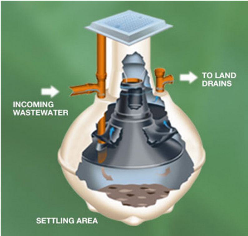
Figure 1.2. Septic tank cross section; (c)Southern Drainage 2007
