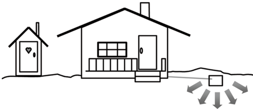
Figure 2. A separate dry toilet and washing waters being led to the ground. This solution is possible only if the amount of washing waters is not great. (Tuukkanen 2006)
