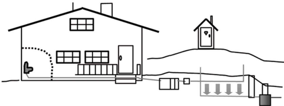
Figure 5. All wastewaters are treated in a buried sand filter equipped with a separate unit for phosphorus precipitation (Tuukkanen 2006).
